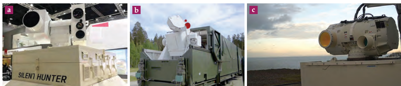
FIGURE 3. NON-US SYSTEMS. (a) China's Silent Hunter laser weapon is housed in a transportable container. Apertures contain the high-energy laser, tracking sensors, and illuminating lasers. (Courtesy of the Defense Systems Information Analysis Center.) (b) Russia's Peresvet “dazzler” weapon is mounted atop a transportable military container. The white beam director rotates about two axes to track a target in space. (Courtesy of the Russian Ministry of Defense, CC BY 4.0 DEED.) (c) The Dragonfire laser 8 is the UK's demonstration of a high-energy laser weapon. The larger aperture houses the weapon's beam director, and the smaller aperture houses a tracking sensor. (Courtesy of MBDA.)
